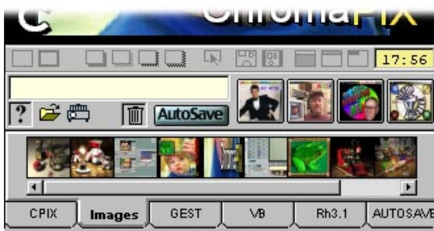
The image storage system used in ChromaPIX is based on drag and drop loading and saving and the use of six thumbnail based image trays. To load an image from a disk file simply select the desired directory from the directory tabs along the bottom edge and then click and drag the image thumbnail from the image tray onto the main image window. To save an image drag from the main image window onto one of the six image trays.
